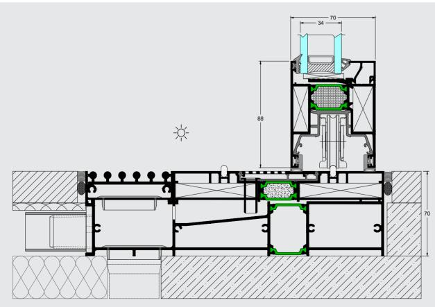
Flat bottom track - water drainage system
