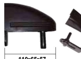
Made of steel and zinc, coated in black. Plastic cover and stainless steel pin φ12, Y 35mm. Adjusts horizontally 40-80mm and vertically 15mm.
