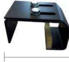
Made of galvanised steel and coated in black colour. Adjusts in horizontal and vertical dimensions. The add of the teflon on the lower side, gives proper alignment, smooth rolling and continuous hold of the gate in order to prevent troubles in functionality.
