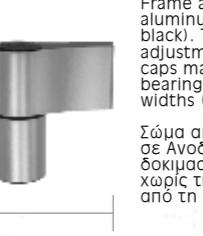
Frame and sash part made of high quality extruded aluminum. Available in 2 colors (Anodized and 9005 RAL black). Tested for 200,000 cycles. CE Certified. Easy 3D adjustment, no need to lift or take out the sash. End caps made of ASA, UV resistant plastic. Sliding plastic bearing to ensure proper operation of the hinge. 2 widths (60mm, 67mm).
