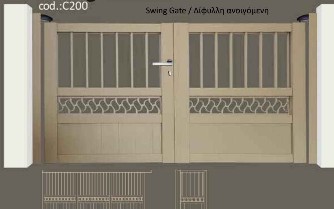
**C200** The design is traditional. The lower part is matchboard of 130x14mm. The decoration is aluminum sheet formed in laser. The upper part of the gate is made with 14x14mm in vertical alignment.
