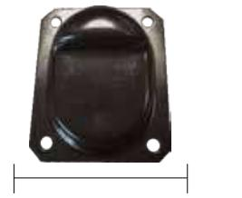
Travel stop for side-hung gates. It is fixed with plugs and is combined with a bolt to secure the gate. It is made of electrogalvanised steel and it has 4 points of fixation.
