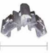
Aluminum corner joint for the "Prestige" Product Line. The large size and the special section achieve maximum robustness and enables us to construct large gate dimensions. The corner joints are from the Italian firm Comunello. They are made of aluminum with stainless steel screws to prevent oxidation.
